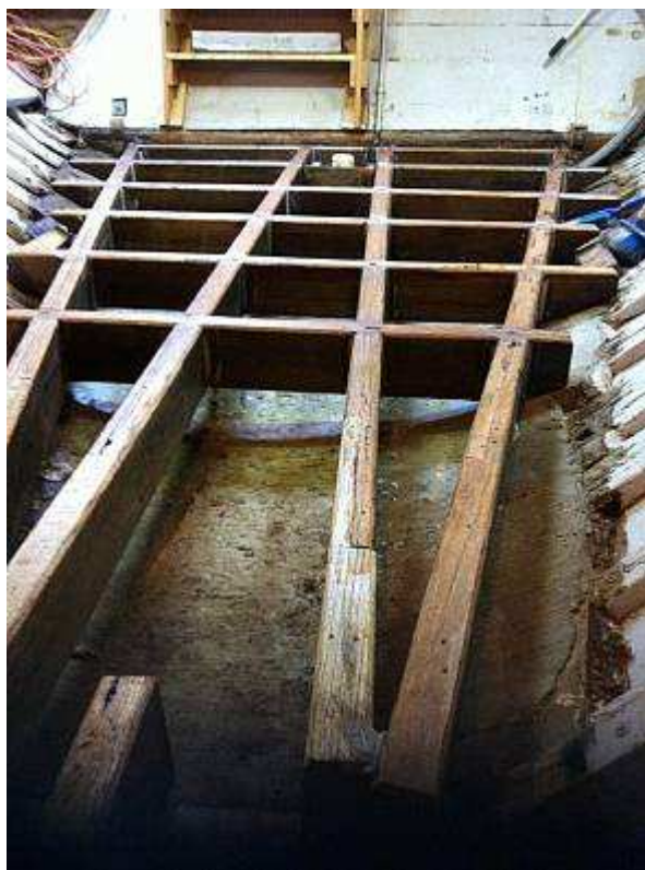
New sub-floor bearers were installed to support a new floor. The original 1915 layer of concrete on the hull was in good order.
