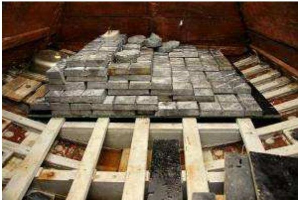
Five tonnes of lead ballast was needed in the well to compensate for increased buoyancy
