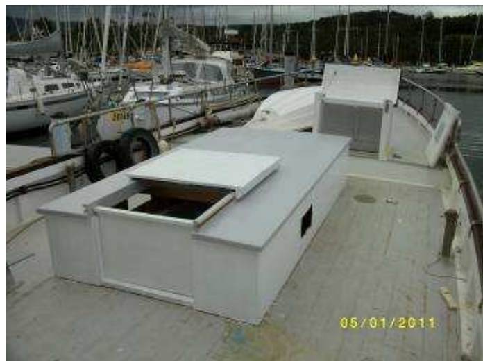
The new deckhouse over the well. Windows are yet to be put into the sides.
