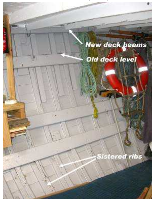
Inside the fo'c'sle, showing new ribs to support the raised deck
