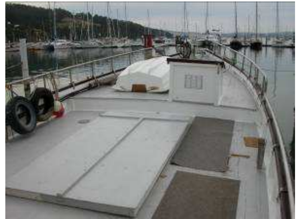
The forward deck was raised by three planks in 1964
