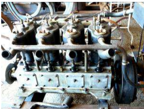
Napier engine, 4 cylinder dual ignition truck engine in Finlay Museum, NSW. Photo thanks to Howard Barber
